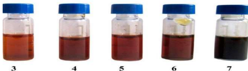
1 – boshlang'ich, 2 – 100 °C (1 soat), 3 – 120 °C (1 soat), 4 – 140 °C (1 soat), 5 – 150 °C (1 soat), 6 – 140°C (2 soat), 7 – 140°C (5 soat) da 3–rasm – [BMIM][Cl] ning harorat va issiqlik bilan ishlov berish davomiyligi oshishi bilan rangi o'zgarishi melanoidin hosil bo'lishi va suvsizlanishi.
