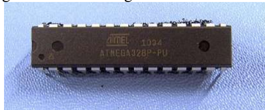
1-rasm. Atmega328 mikroprosessori ko‘rinishi.
