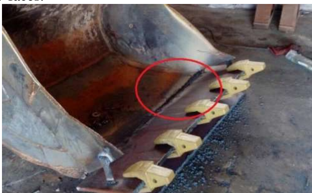
Figure 3: Defect resulting from plate separation from the jaw part of the bucket
