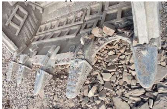
Figure 4: Backhoe bucket jaw plate defect
